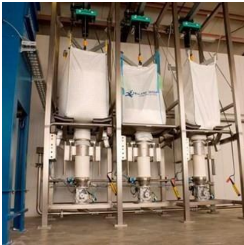
Big Bag losinstallatie
